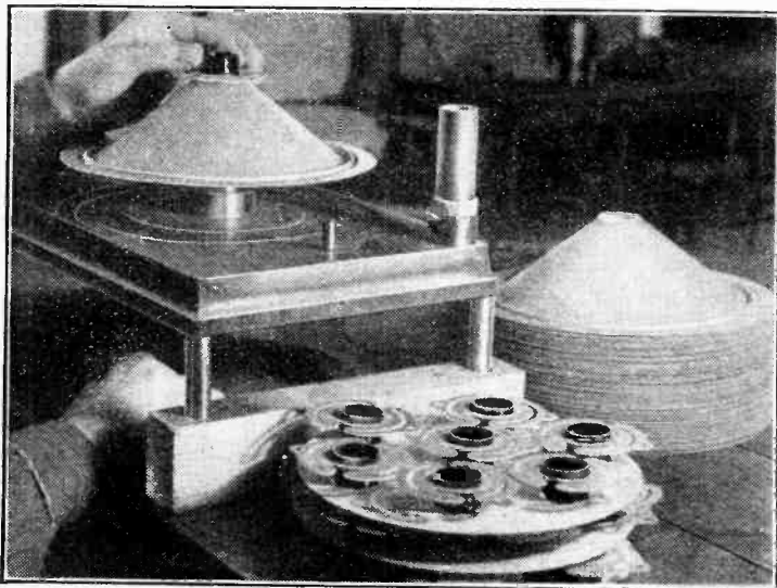
LOUD SPEAKERS IN THE MAKING. A photograph taken in a factory showing a moving-coil being fitted in position.
